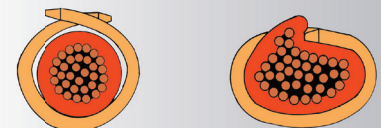
Insulation is not securely held
